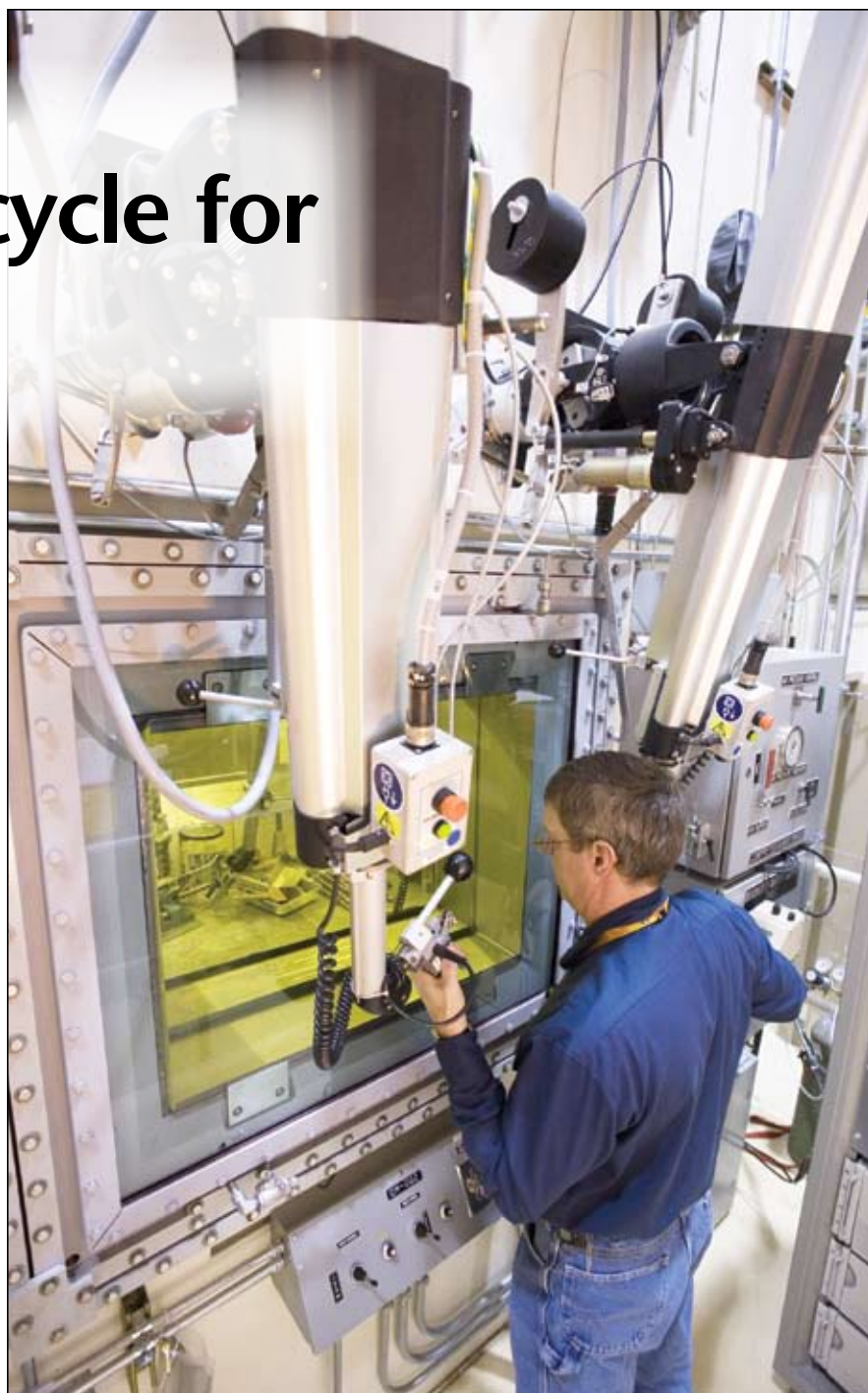
Michael Connors of Inorganic Isotope and Actinide Chemistry uses the hot-cell manipulators in the Laboratory's Isotope Production Facility at the Los Alamos Neutron Science Center. Photo by LeRoy N. Sanchez, Records Management/Media Services and Operations
