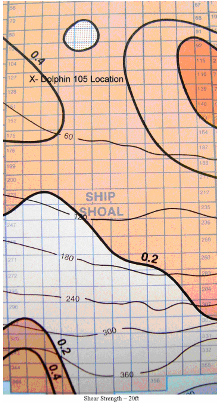
Figure 22: Soil Shear Strength at Dolphin 105 Location
