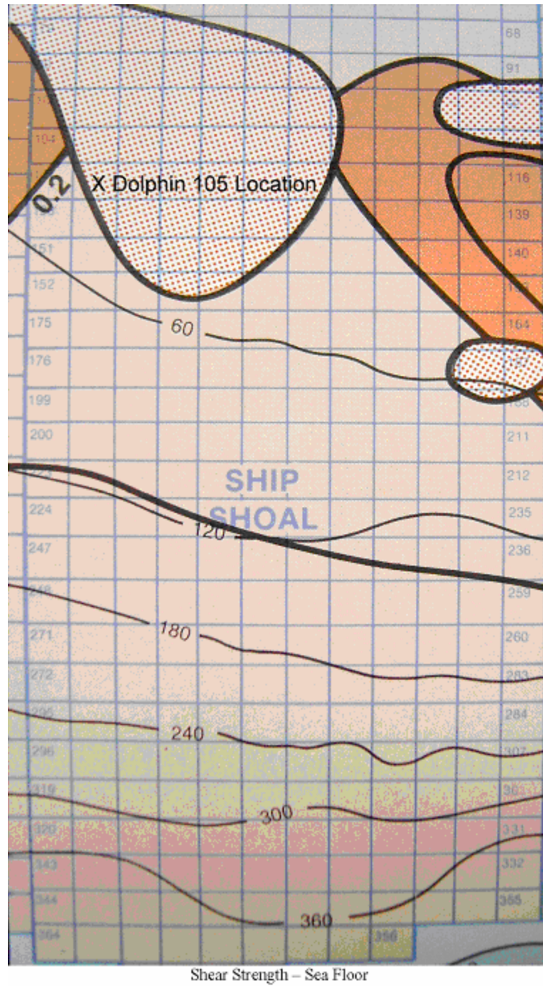
Figure 21: Soil Shear Strength at Dolphin 105 Location
