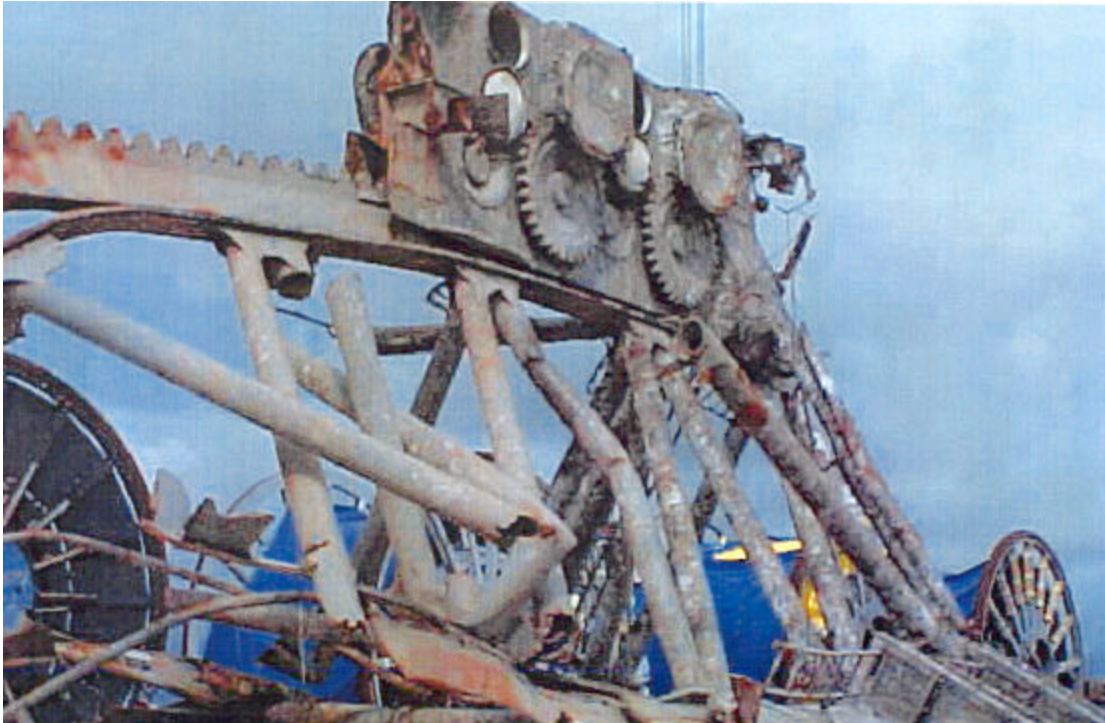
Figure 34: Starboard leg recovered showing gear train still attached.
