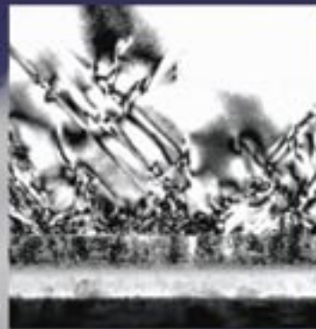
Transmission electron micrograph showing a cross-section of ACSi film and underlying buffer layers on metal tape.
