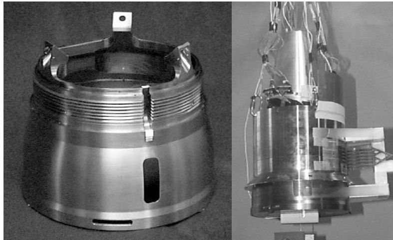
Figure 1: Titanium Mount (left) and Experimental Test Configuration (right)
