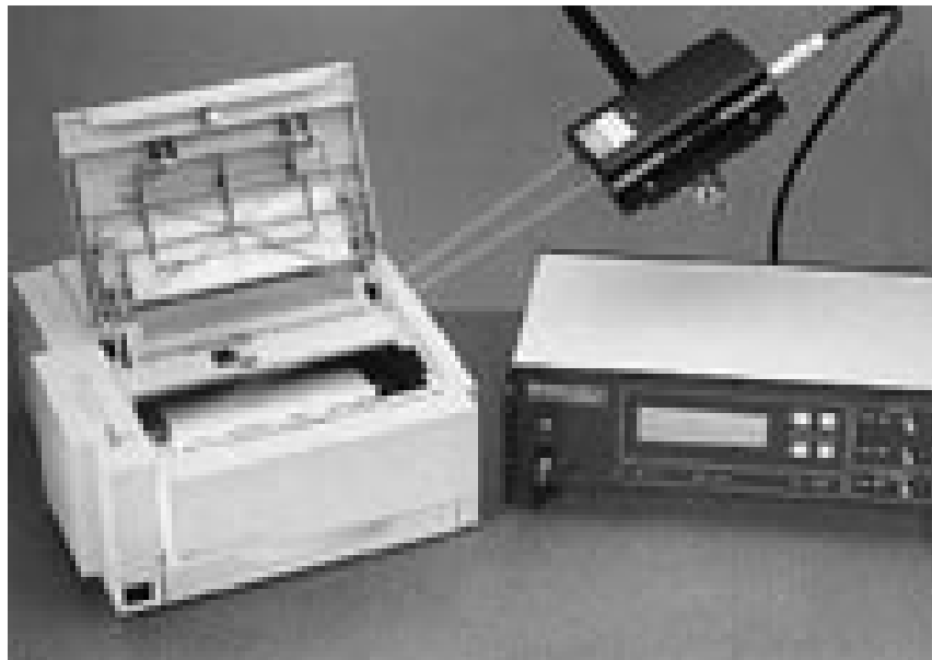
Figure 7. In-plane measurement on a printer drive using a laser Doppler vibrometer. The LDV permits velocity or displacement measurements of hot, miniature or soft surfaces, even under water, without mass-loading. (Courtesy of Polytec, Inc.: www.polytec.com )
