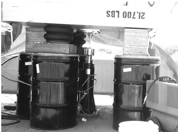
(a) A hydraulic shaker: larger force capacity than electrodynamic shaker but limited high-frequency capability.
