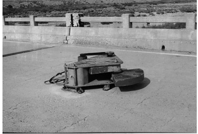
(b) Mechanical eccentric mass shaker: generates sinusoidal excitation, but difficult to apply in vertical direction.
