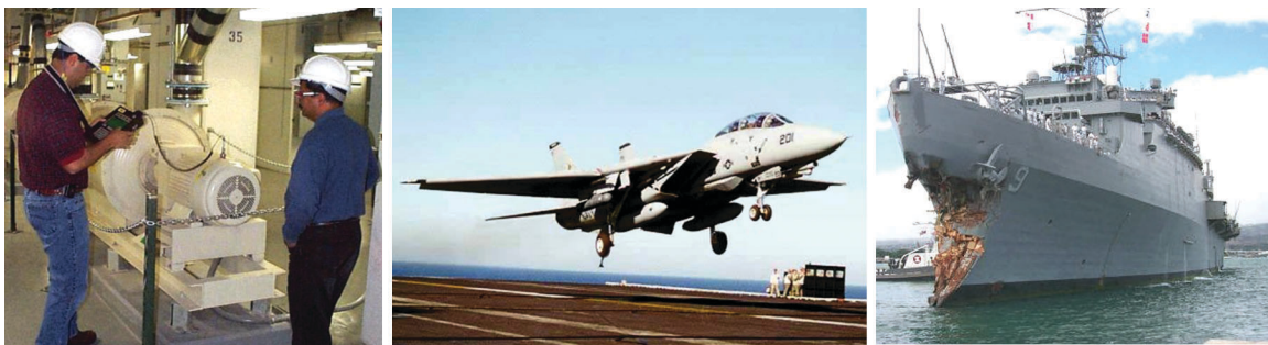
Figure 5.1 Illustration of three categories of damage. From left to right, (a) incremental damage accumulation in rotating machinery, (b) scheduled discrete damage accumulation resulting from an F-14 Tomcat landing on a carrier, and (c) unscheduled discrete damage accumulation resulting from a collision of the USS Denver.
