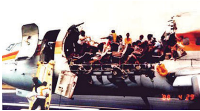
Figure 1.7 Damage to Aloha Airline fuselage resulting from fatigue cracks.
