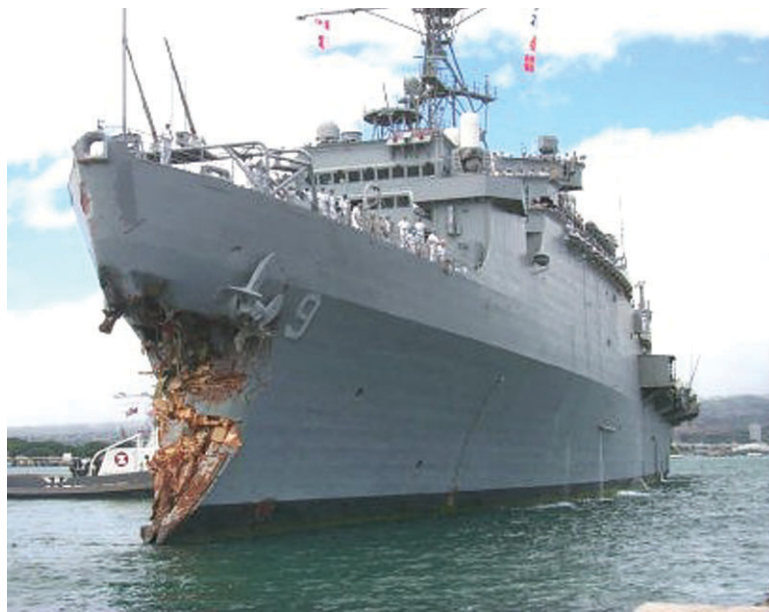
Figure 1.2 Damage to the USS Denver.
