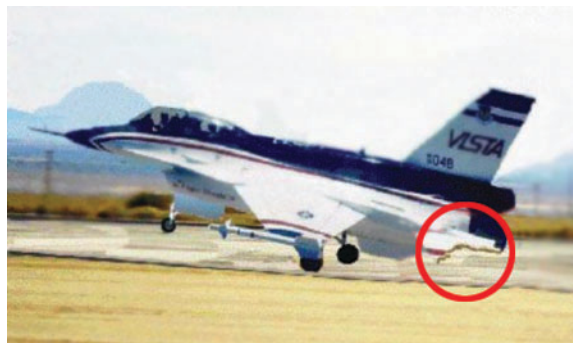
Figure B3 Vista F-16 with a failed left-side stabilator landing successfully with the use of reconfigurable control.
