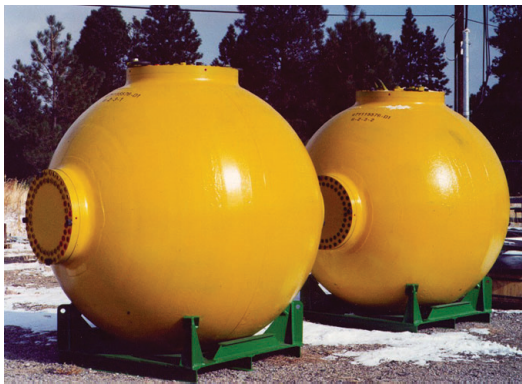
Figure B4 Explosive-containment pressure vessels. Figure B5 Results from a high-fidelity finite-element (FE) model.
