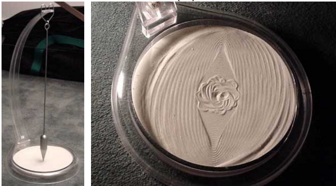
Fig. 12: Records of the February 28, 2001 Earthquake at Olympia, Washington. (Top: Time-domain signal. Bottom Left: Sand-tracing pendulum. Bottom Right: Patterns produced by the pendulum. The pendulum performs a transform of the original signal analogous to phase-amplitude decoupling. A steady-state periodic signal produces the circle-like pattern seen on the outside. The transient Earthquake signal produces the twisted pattern at the center.)
