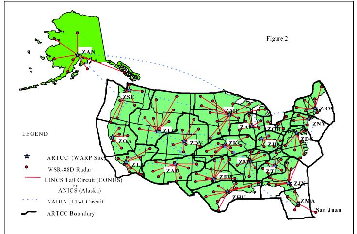
**Figure 2** - WSR-88D connections to WARP within each ARTCC. Every CONUS network WSR-88D is connected to at least one WARP.
