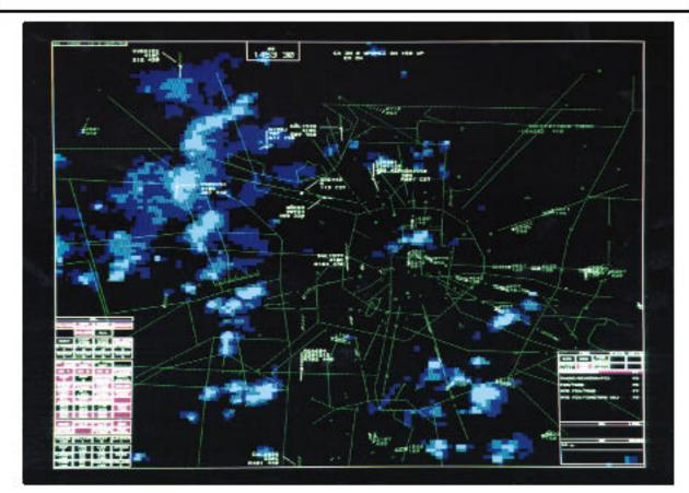
Figure 3. Example of en route air traffice controller's display. The reflectivity source is the WSR-88D via the pathway and systems shown in Figure 1. Aircraft target information comes from the Air Route Surveillance Radar (ARSR) system. Other lines and characters are jet routes and navigational aid positions. The box in the upper left contains elements for the air traffic controller to reconfigure his display (see text for further information).
