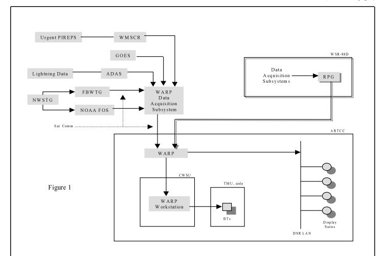
**Figure 1** - WARP, Stage 1/2 configuration showing data sources and sinks. Notice that WARP, Stage 1/2 has Associated PUP connections to WSR-88Ds and a direct connection to the air traffic controller's display system, the latter for the purpose of delivering four WSR-88D reflectivity products.
