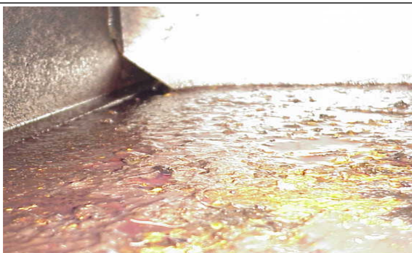
A tank infected with a fuel fouling fungus.
