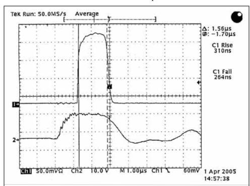
**Figure 1:** Detected pulse resulting when the transmitter is brought up with all cavities set to data sheet values.
