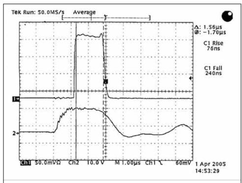
**Figure 3:** Detected pulse with cavity 4 set too low.
