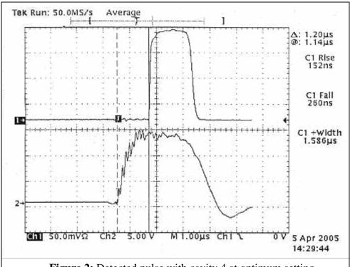
Figure 2: Detected pulse with cavity 4 at optimum setting.
