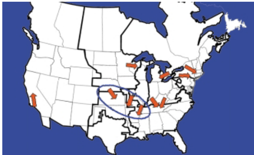
Figure 7-2 Current Electric Power Bottlenecks
