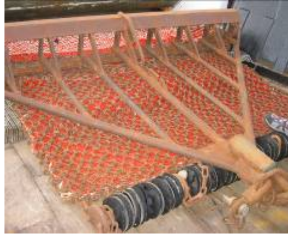
Mesh netting in the dredge
