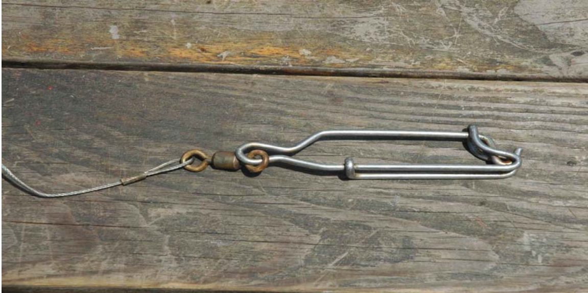
Gangion clip attached to 20 foot line with hook (Circle or J) and Pacific Mackerel bait.
