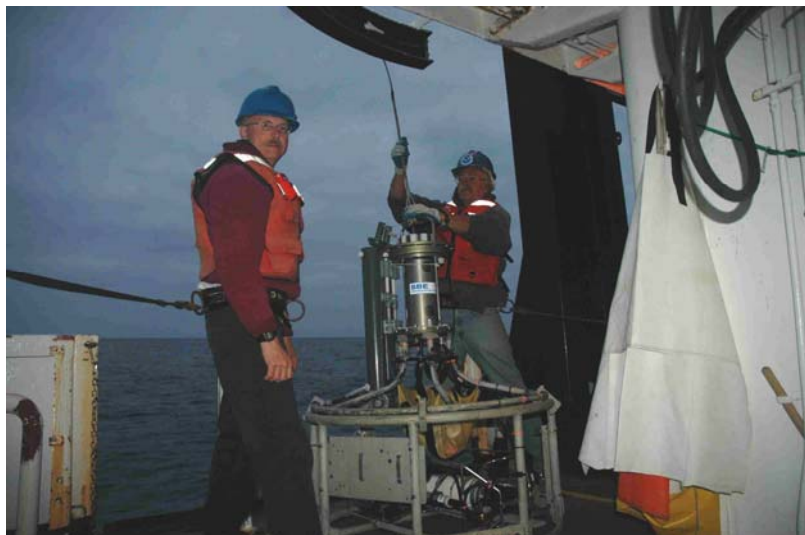
NOAA scientists, Eric Lynn and Dr. Russ Vetter prepare to lower the CTD. Notice the green cylinders on the left side of the CTD – they are bottles for water samples.
