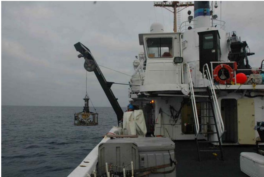
The CTD being lowered from the J Frame on the NOAA ship DAVID STARR JORDAN
