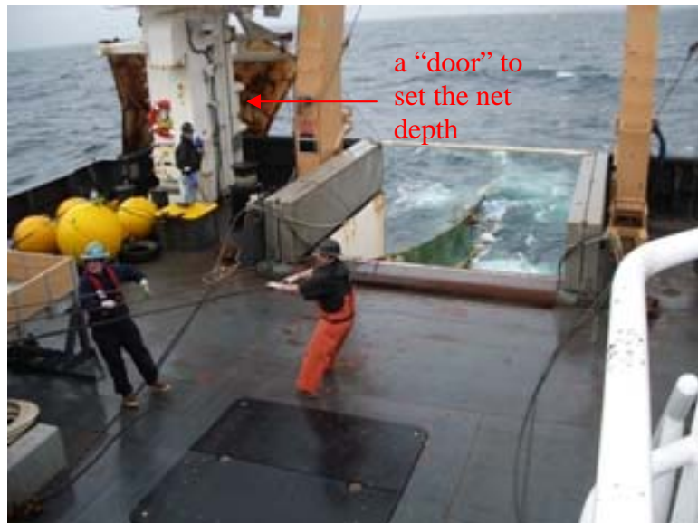
The fishing and deck crew of the OSCAR DYSON release the net for a trawl sample.
