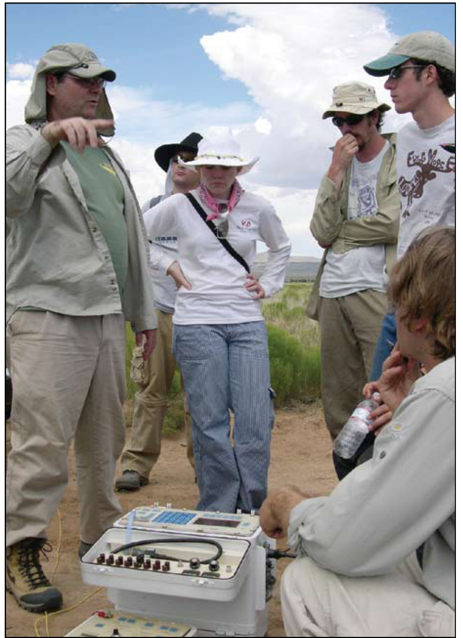
Scott Urquhart, left, of Zonge Engineering and Research Organization Inc. explains to students in the Summer of Applied Geophysical Experience (SAGE) program how to perform transient electromagnetic sounding to determine the depth to ground water. SAGE is an educational program designed to introduce students in geophysics and related fields to “hands on” geophysical exploration and research. Photos by Caryn Johansen
