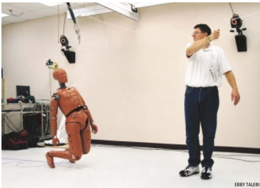
Shawn Applegarth, a mechanical engineer, and other investigators at the James A. Haley Veterans' Hospital's Patient Safety Center, recently completed a preliminary study on fall-related injuries using a car crash test dummy as the subject. The investigators are hoping to learn more about the human body's reaction to a serious fall and how new and emerging technologies may prevent serious injuries to those at risk for falls.
