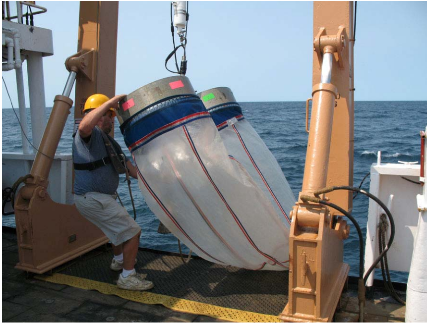
A crewmember bringing in the CTD and Bongo Nets after sampling
