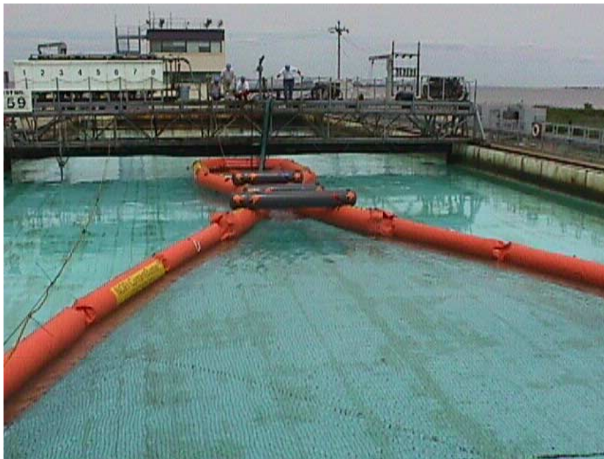
Figure 6-4. NOFI Current Buster™ in Ohmsett tank.
