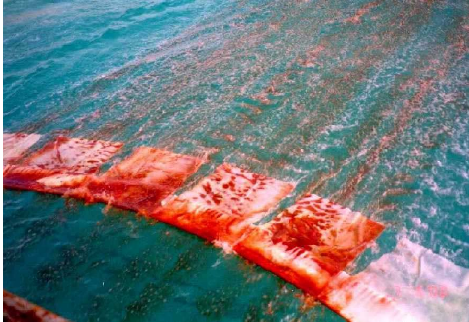
Figure 7-4. Sheet absorbents at 3.5 knots.
