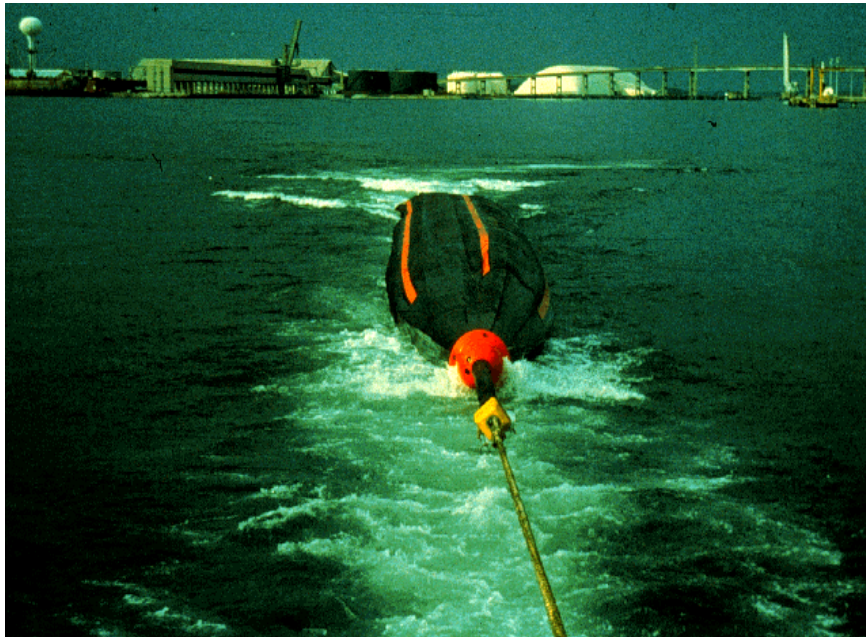
Figure 8-13. Sea slug barge floating bladders.
