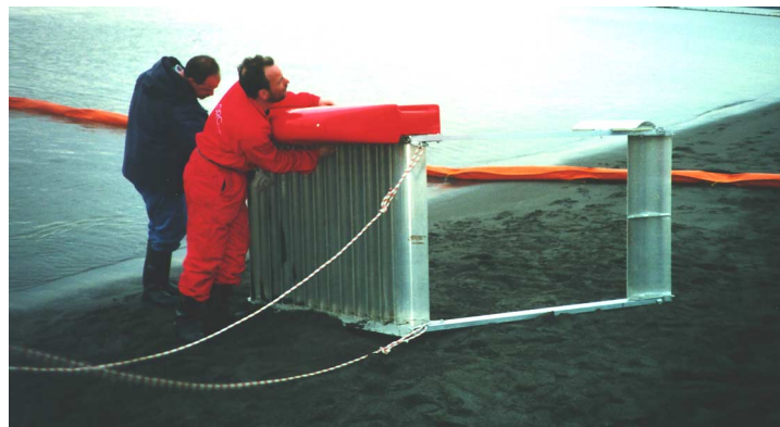
Figure 5-8. Boom vane is quickly assembled.
