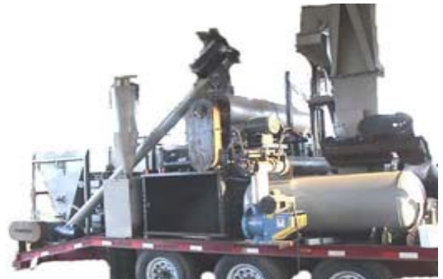
Figure 2. Renewable Oil International portable pyrolyzer.
