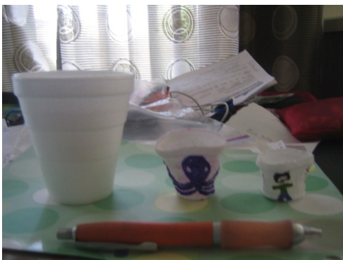
This is a “regular” Styrofoam 10 oz cup and the two cups that returned from -4500 meters. The far right cup has a Flat Stanley drawn on it.
