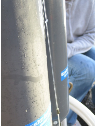
The bottles on the CTD rosette. In the foreground is the bottle containing 4380 meter water at 1.518 degree water, the background contains the water from near the surface at 14.169 degrees.
