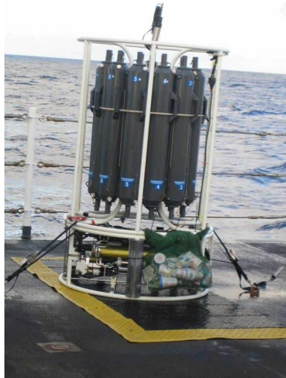
The CTD on the fantail of the MCARTHUR II with Styrofoam cups in the green mesh bag for the second deep cast of -4500 meters.
