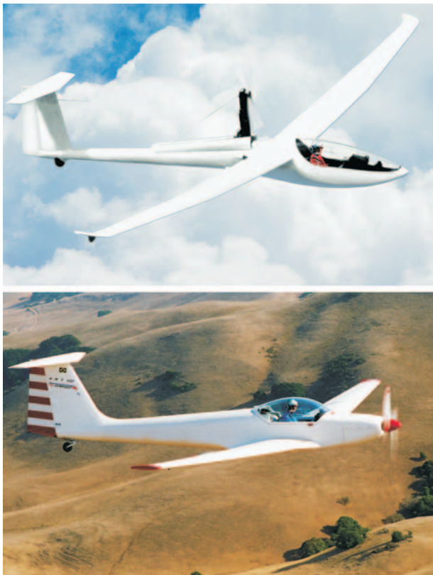
Figure 7-24. Types of self-launch gliders.
