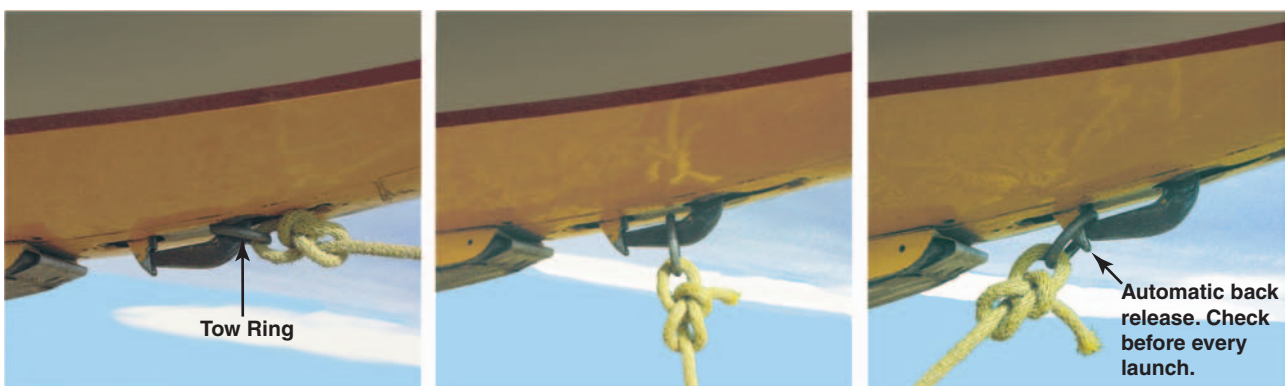
Figure 7-13. Testing the towhook.
