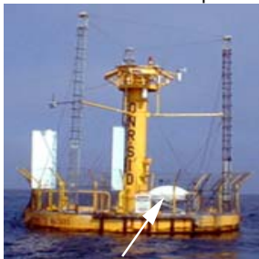
First test of a radar wind profiler on a 10-m discus buoy
