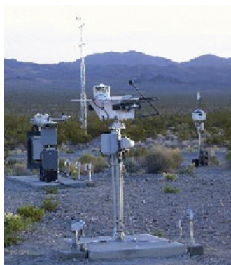
Instrumentation at the Desert Rock, NV site of the ARL SURFRAD program. SURFRAD is the Nation's surface radiant energy balance monitoring network.
