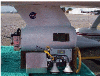
The ARL instrumentation pod mounted beneath a light aircraft, and showing the Ka-band scatterometer normally used for studies of air-sea interaction and surface waves.
