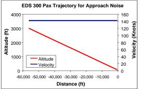
Per certification procedures, Approach noise is calculated at approach speed + 10 kts
