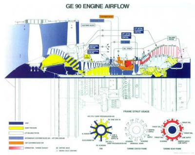
A cross-section of a particular engine can be used to calibrate locations and dimensions
