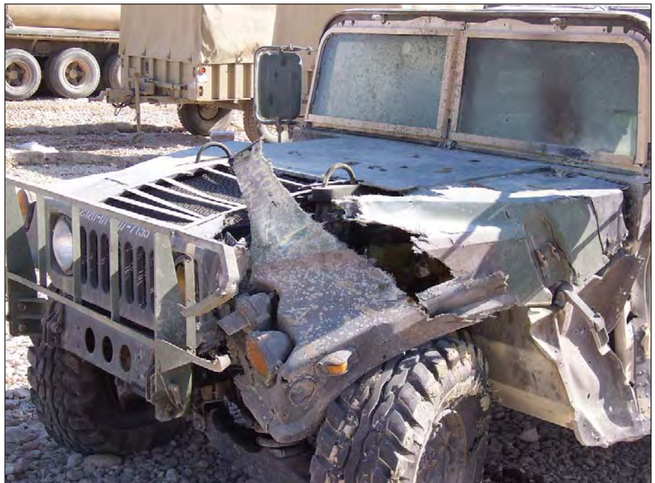
U.S. Marine Sergeant Luke Cassidy was driving this Humvee when an improvised explosive device (IED) detonated underneath the front driver's side wheel destroying the front left axel of the vehicle.
