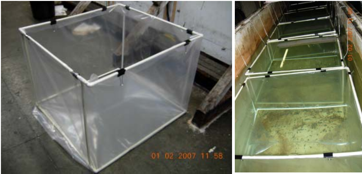
Figure 90. Construction and Installation in Tank of Cells for Evaporation in Ice Experiments
