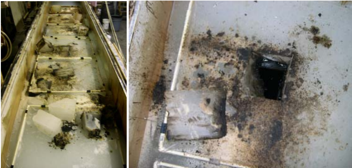
Figure 91. Extraction of Oil Samples for Evaporation Analysis after 50 Days Encapsulation
