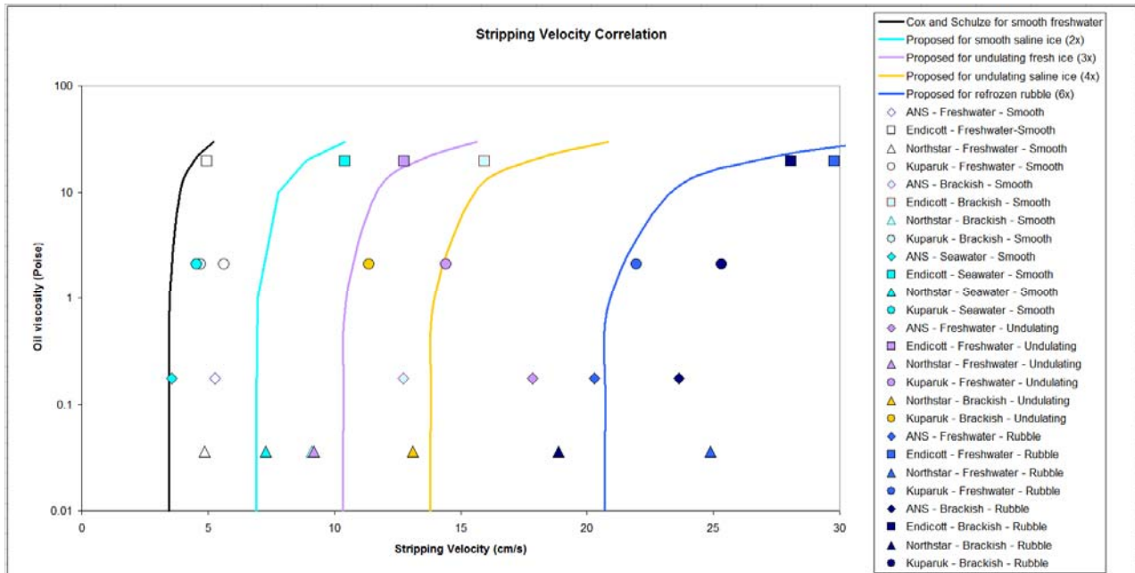
Figure 59. Comparison of Equation 20 Predictions with Experimental Data (after Cox and Schultz 1986)
