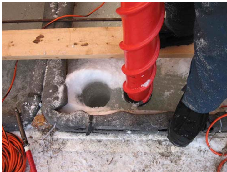
Figure 88. Extracting Cores from the Outdoor Test Tanks
