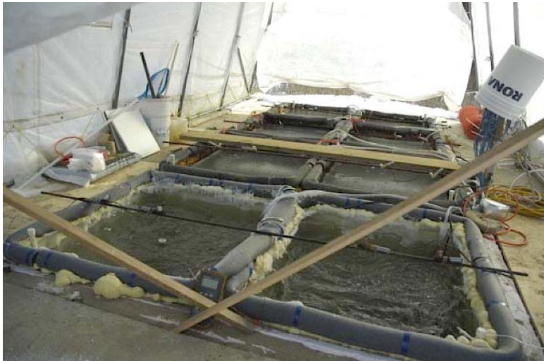
Figure 85. View of All Eight Tanks as Utilized During the Winter 2006/07 with Two New Tanks Added After the First Year to Incorporate the Sediment Add-on
