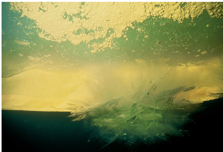
Figure 83. Underwater Photograph Showing Extremely Fragile Frazil Ice Crystals Hanging Beneath Fast Ice During an Experimental Spill of Emulsified Oil (visible hanging below the ice in the background) Large partly agglomerated drops of emulsified crude are visible in the foreground Source: Buist et al. (1983)
