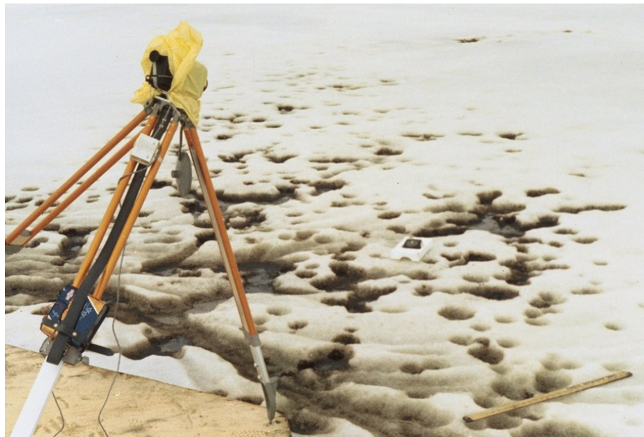
Figure 81. Initial Surface Appearance of Crude Oil Migrating Through the Ice at the Dome Oil and Gas Under Sea Ice Experiment in Early June 1980
