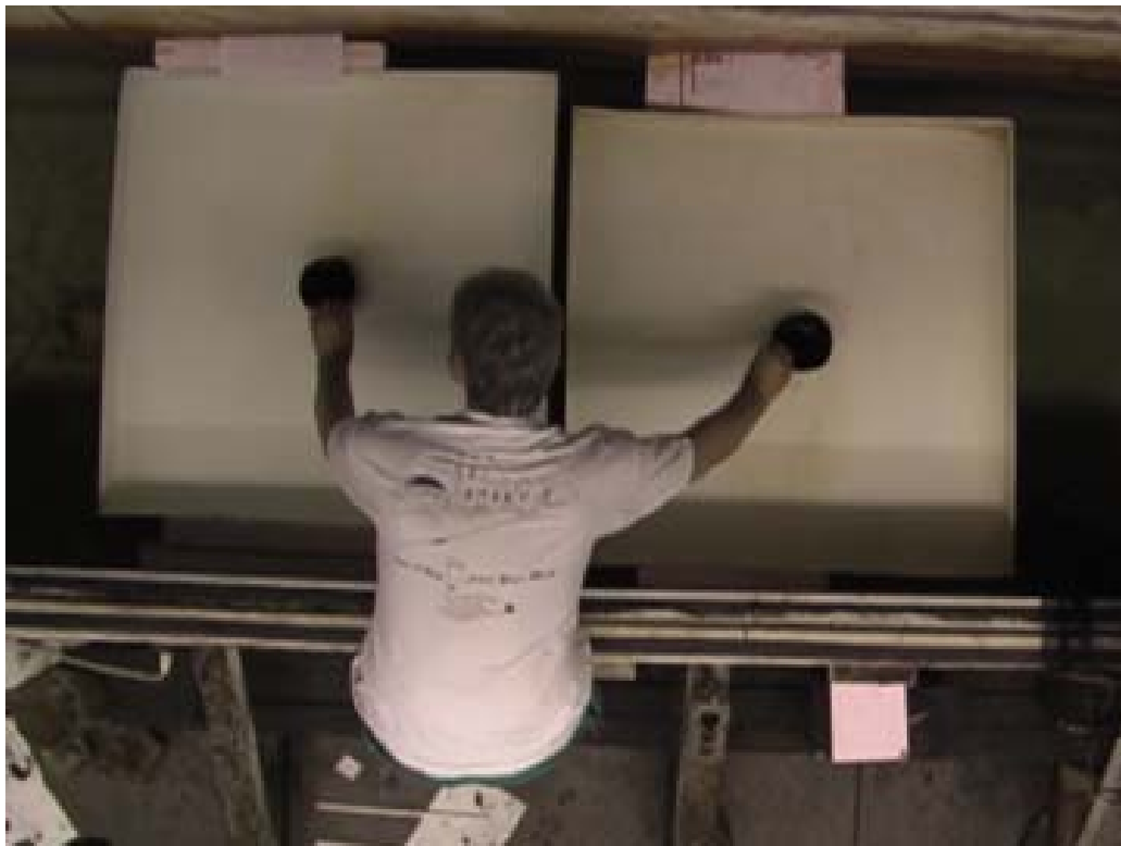
Figure 14. Releasing Oil by Hand from Metal Rings in Center of Pans
