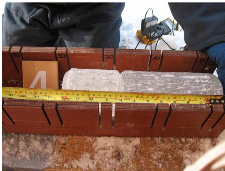
Figure 89. Example Ice Core #4 Extracted from Tank #3, 30‰ Water
