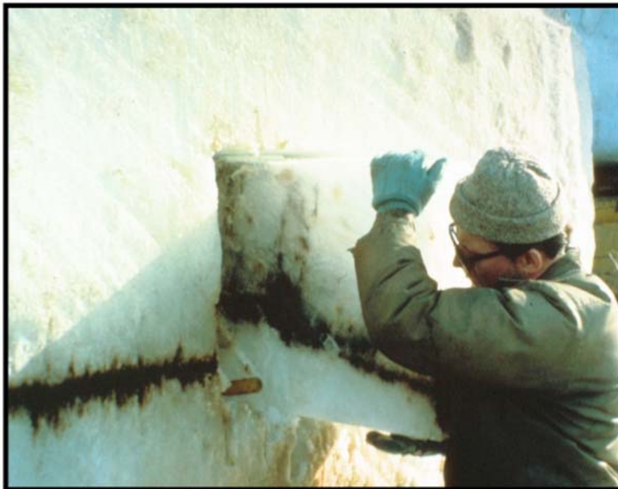
Figure 80. Trapped Oil Lens Visible in a Large Block of Sea Ice Cut Out of an Experimental Spill in Alaska Photo: A. Allen
