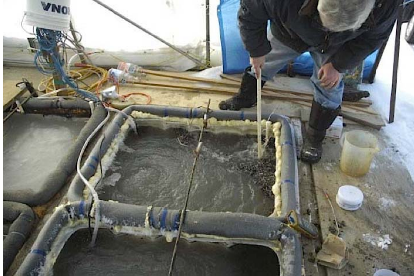
Figure 86. Mixing Sediment into Agitated Tanks Prior to Adding Snow
