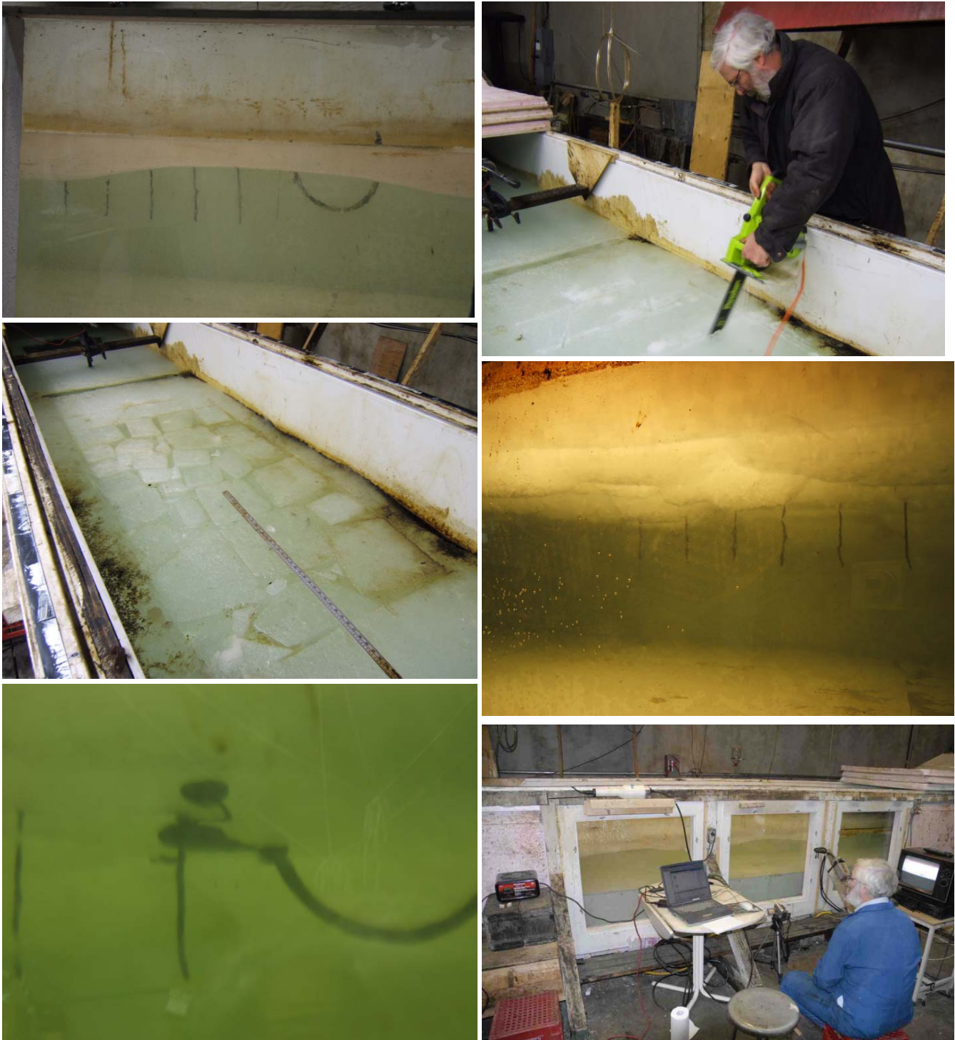
Figure 56. Various Ice Sheets Used in Experiments on Oil Movement Under Ice
