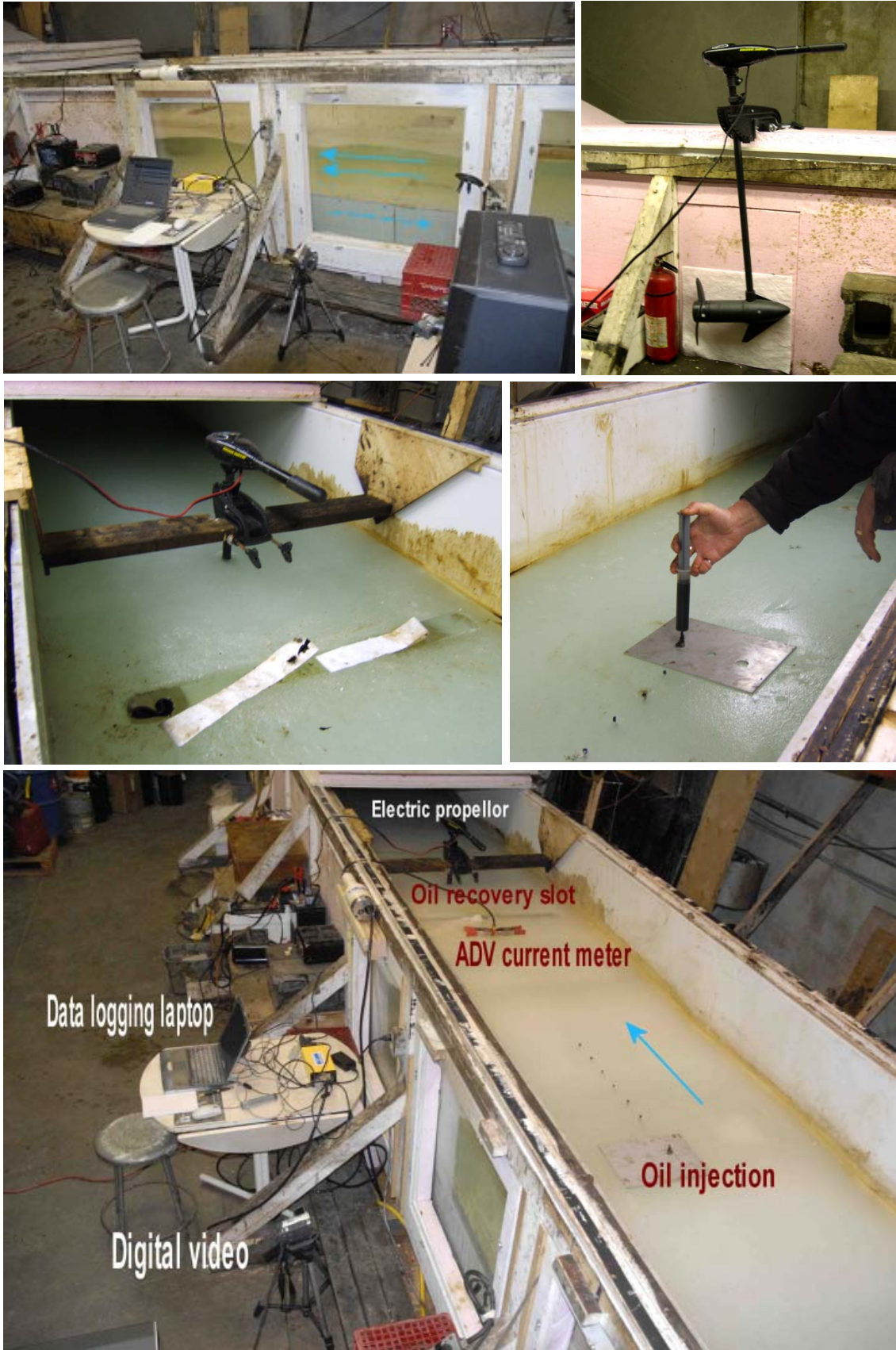
Figure 55. Indoor Tank Setup for Oil Movement Under Ice Experiments
