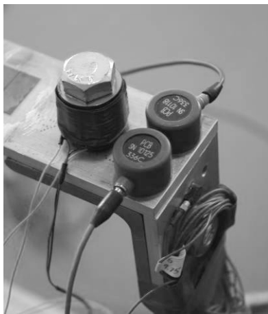
Figure 21 - Two accelerometers were placed side by side on the test structure. The closer accelerometer is attached to the Husky system, while the far accelerometer is attached to a commercial data acquisition system.
