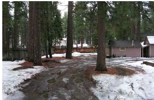
Unpaved driveways may contribute significant sources of sediment, oil and grease to stormwater runoff that eventually reaches Lake Tahoe.
