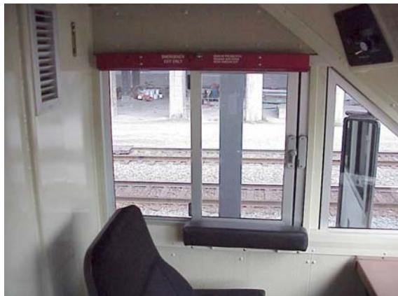
Figure 3. Interior view of F59 cab emergency exit window
