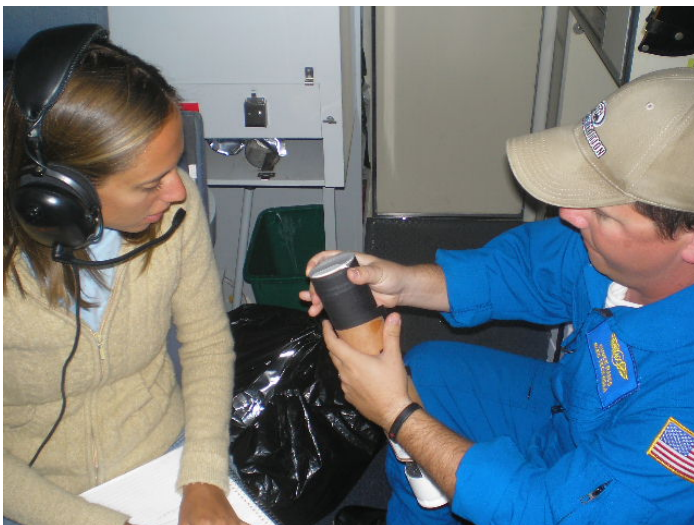
Electronic Technician, Chuck Rasco, explains to me how to prepare a dropsonde for the next drop.
