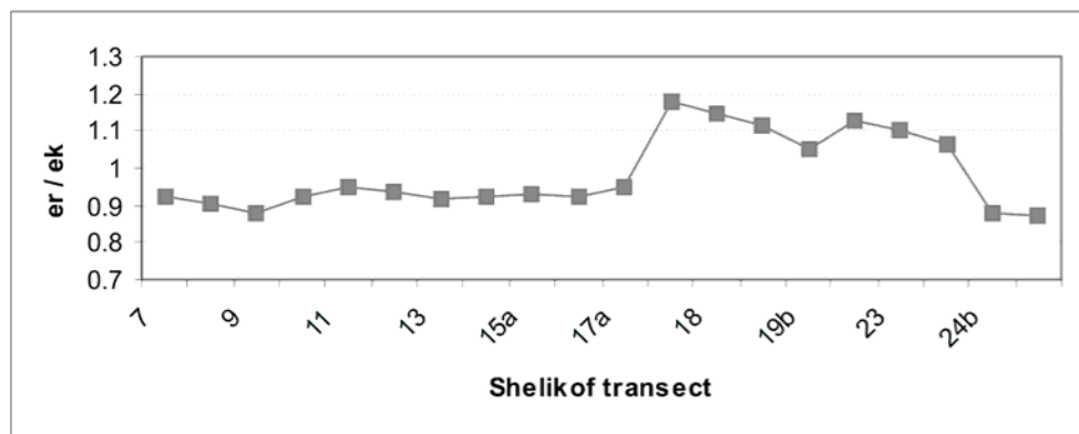
Figure 8. Ratio of mean s_A at 38 kHz from the EK500 (ROMS 5.30) and ER60 (V2.0.0) for transects conducted in Shelikof Strait. Note the dramatic increase in s_A ratio along transect 17 and dramatic decrease along transect 24. [Figure courtesy of N. Williamson]
