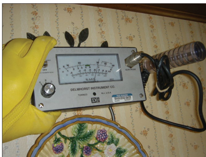
Figure 3a. An intrusive/penetrating moisture meter—recommended for final moisture readings.
