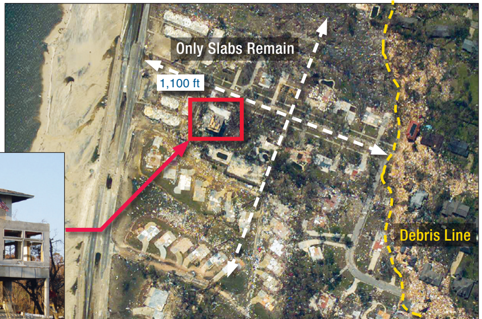
Figure 13. Pass Christian, Mississippi, home elevated on reinforced concrete columns in Zone A, with the bottom of the floor beam elevated approximately 9 feet above the BFE. Although Katrina flooding was approximately 4 feet above the top of the lowest elevated floor, the home sustained no structural damage. All other buildings in the vicinity were destroyed.
