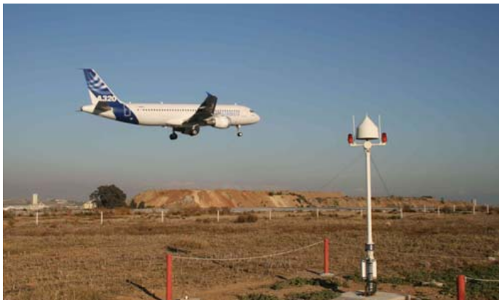
Building momentum for 2008, LAAS closed out 2007 with a successful flight trial in Malaga, Spain. The flight trial was conducted with an Airbus 320 aircraft against a Honeywell SLS-3000 ground station, identical to the one in Memphis. FAA and Spain's Aeropuertos Españoles y Navegación Aérea (AENA) are working closely on implementation of GBAS/LAAS under a cooperative agreement for research and development.
