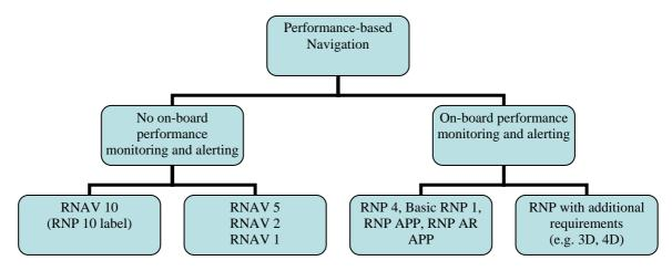
As well as the harmonized navigation specifications, some new navigation specifications were developed for terminal area and approach applications. Work was complete on navigation specifications for RNAV 10 (RNP 10), RNP 4, RNAV 5, RNAV 1, Basic RNP 1, RNP Approach and RNP AR Approach.
