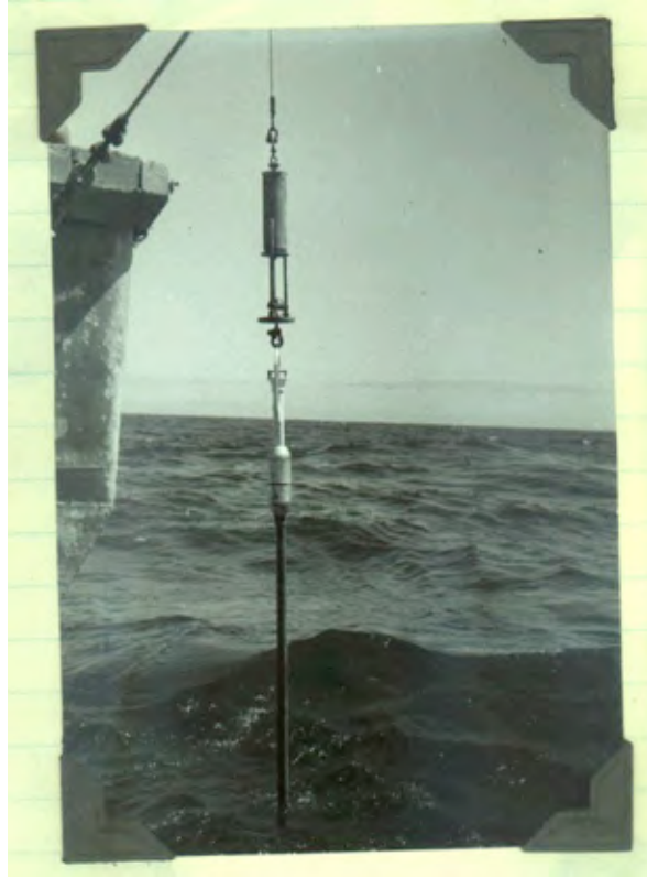
Ball and braker and Pflager Cover ready for lowering.
