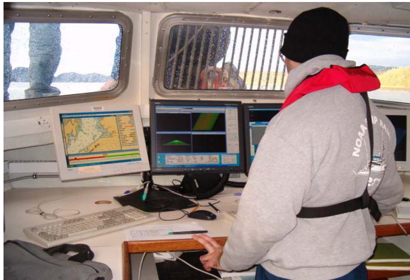
Ensign Stevenson collects multi-beam bathymetric data from the launch
