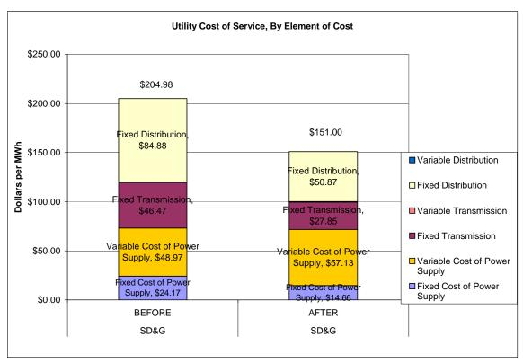
**Figure 6:** Short Run Impact of PHEV Valley-Filling on Components of System Cost for San Diego Gas and Electric
