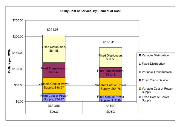
**Figure A.1:** Short Run Impact of PHEV Valley-Filling on Components of System Cost for San Diego Gas and Electric with 60% Market Penetration of PHEVs
