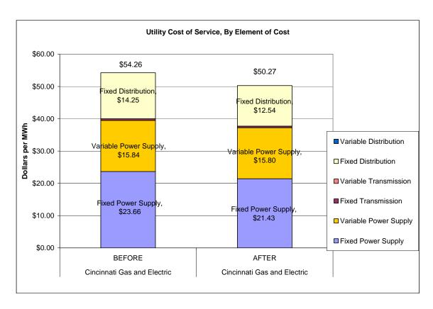
**Figure 4:** Short Run Impact of PHEV Valley-Filling on Components of System Cost for Cincinnati Gas and Electric
