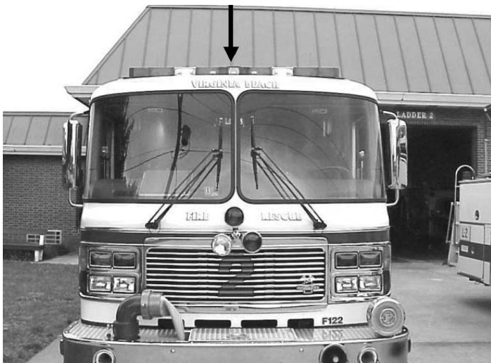
Figure 4-2a. This emitter is mounted within the warning light bar.
