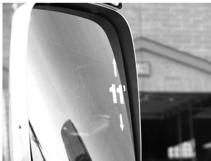
Figure 3-4. Reminding the driver of the vehicle height is important.
