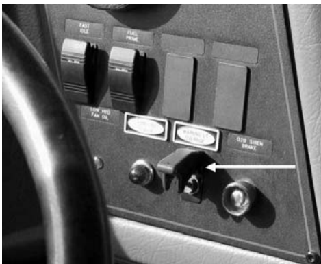
Figure 3-9. The amber lighting override.
