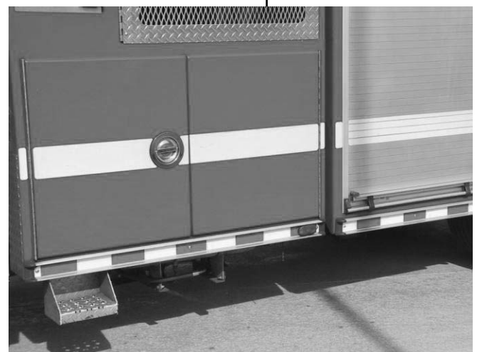
Figures 3-1 a and b. Phoenix fire apparatus have NFPA-required striping and optional DOT-style, red/white truck reflective markings.
