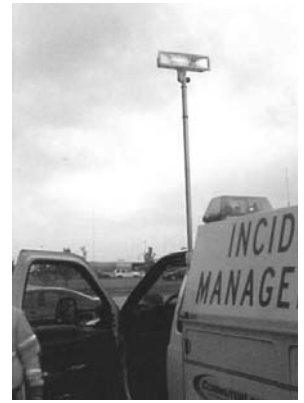
Figure 4-4. A Utah DOT IMT extendable floodlight.
