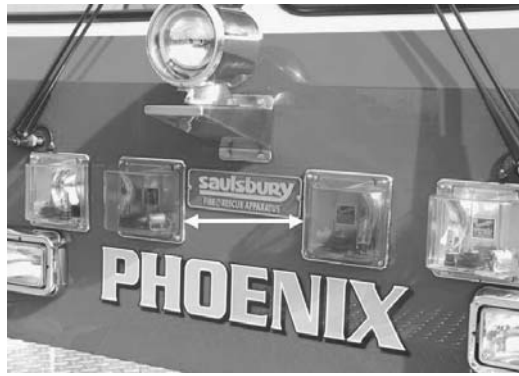
Figures 3-8 a and b. Amber lighting used on Phoenix fire apparatus.
