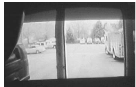
Figure 3-11. The cab-mounted monitor allows the driver to view the area behind the apparatus.
