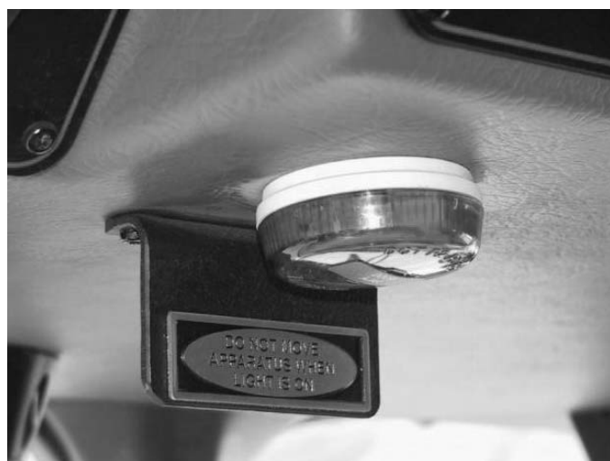
Figure 3-5. The "DO NOT MOVE" light on a Phoenix engine company.
