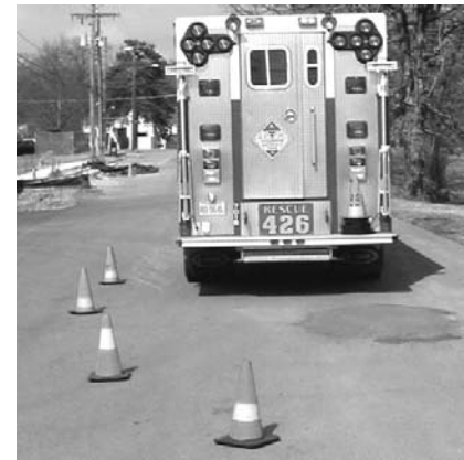
Figure 5-11. A combination of apparatus-mounted warning arrows and traffic cones should be used to redirect traffic.
