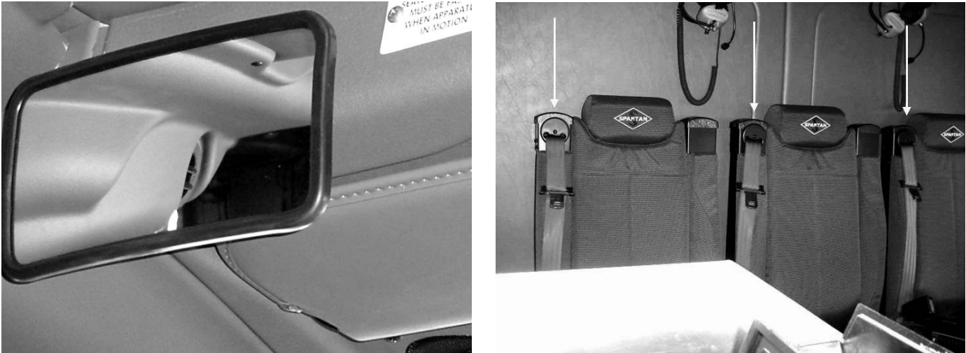
Figures 3-6 a and b. Orange restraints and the officer's seat rearview mirror on Plano fire apparatus.
