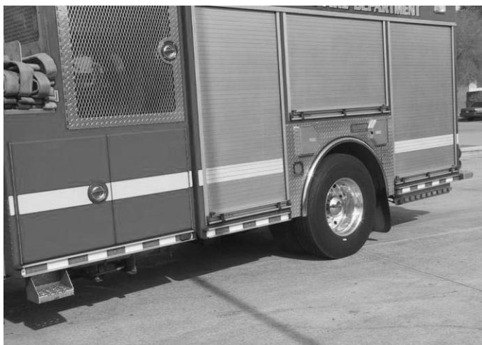
Figures 3-1 a and b. Phoenix fire apparatus have NFPA-required striping and optional DOT-style, red/white truck reflective markings.
