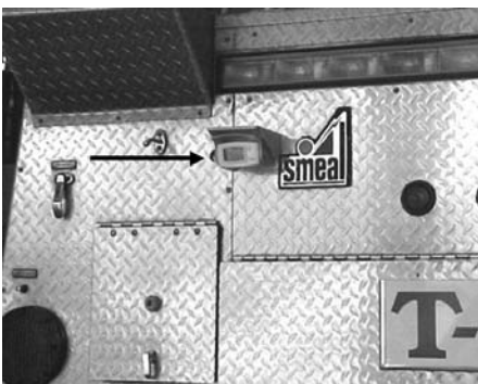
Figures 3-10 a and b. Backing cameras are installed on the rear of the apparatus.
