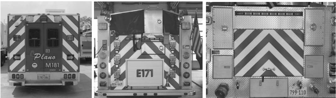
Figures 3-2 a through c. Plano apparatus feature U.K.-style reflective patterns on the rear of the vehicle.
