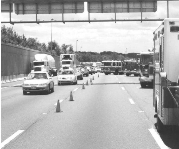
Figure 5-12. Apparatus should be angled at 45 degrees, and cones placed to route traffic around the scene.
