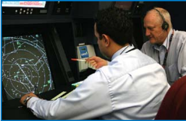
A controller practices radar handoffs at Potomac Consolidated TRACON's simulation laboratory, where the equipment is identical to the systems used on the control room floor. Photo: Jeff Bruzdinski
