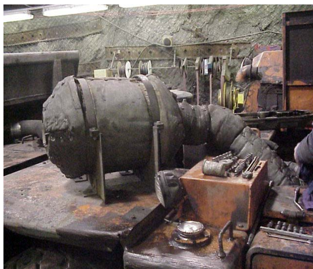
Figure 1. Installation of an Engelhard DPM Filter on a Haul-truck.
