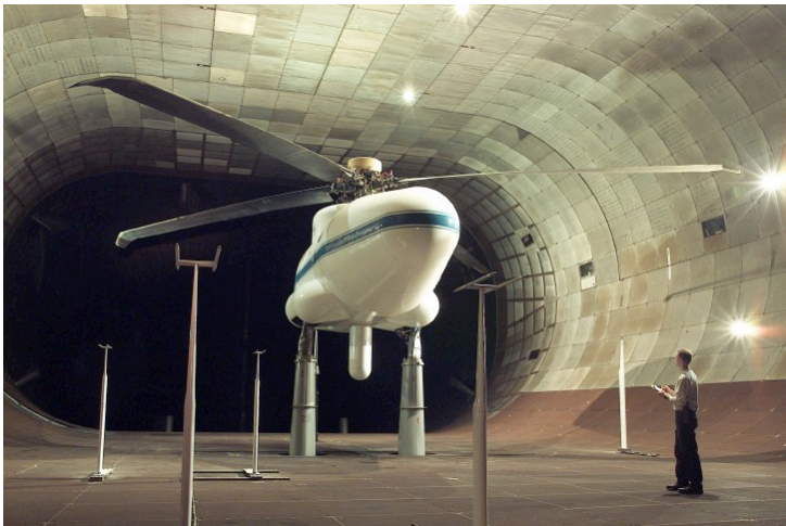
Figure 12. Active Blade Control testing in the NFAC.
