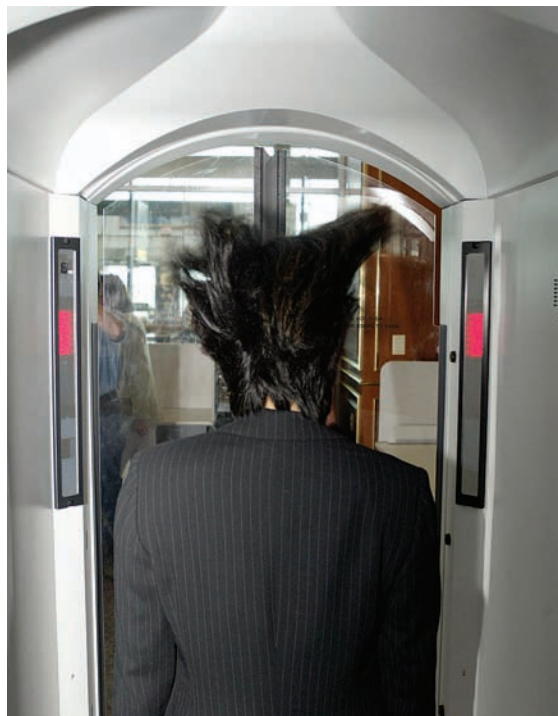
Hair-raising experience? One technology now used for airport security comprises portals in which puffs of air are blown at passengers and then analyzed to detect trace amounts of explosives. THz waves add the advantage of penetrating clothing, and offer a high probability of detection with few false alarms.
