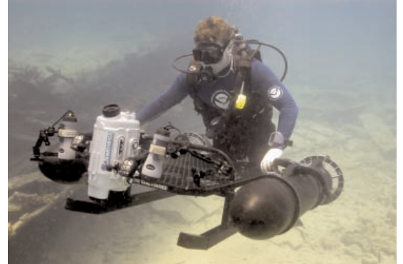
Maritime Archaeologist Tane Casserly operated the propulsion sled to create photo-mosaics of selected Keys' wrecks. Photo credit: Russ Green, Thunder Bay NMS
