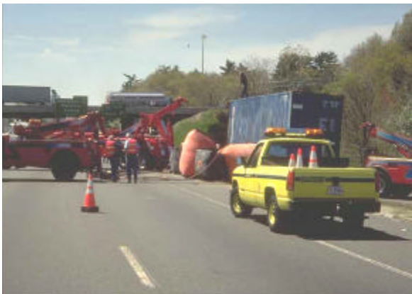
Figure 1-7: DOT operated air-bag being used to up-right tractor-trailer
