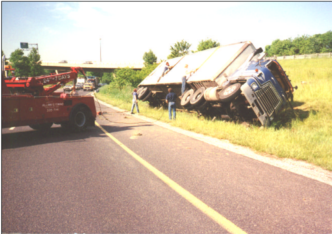
Figure 1-1: Fixed tow-trucks using multiple lanes to upright tractor-trailer
