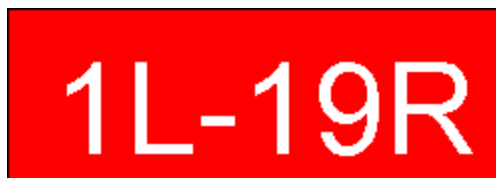
Runway Hold Sign
