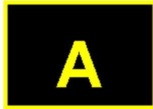
Taxiway Location Sign
