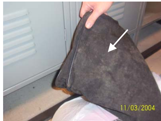
Figure 4. Visible mold on firefighting clothing in turnout gear room.
