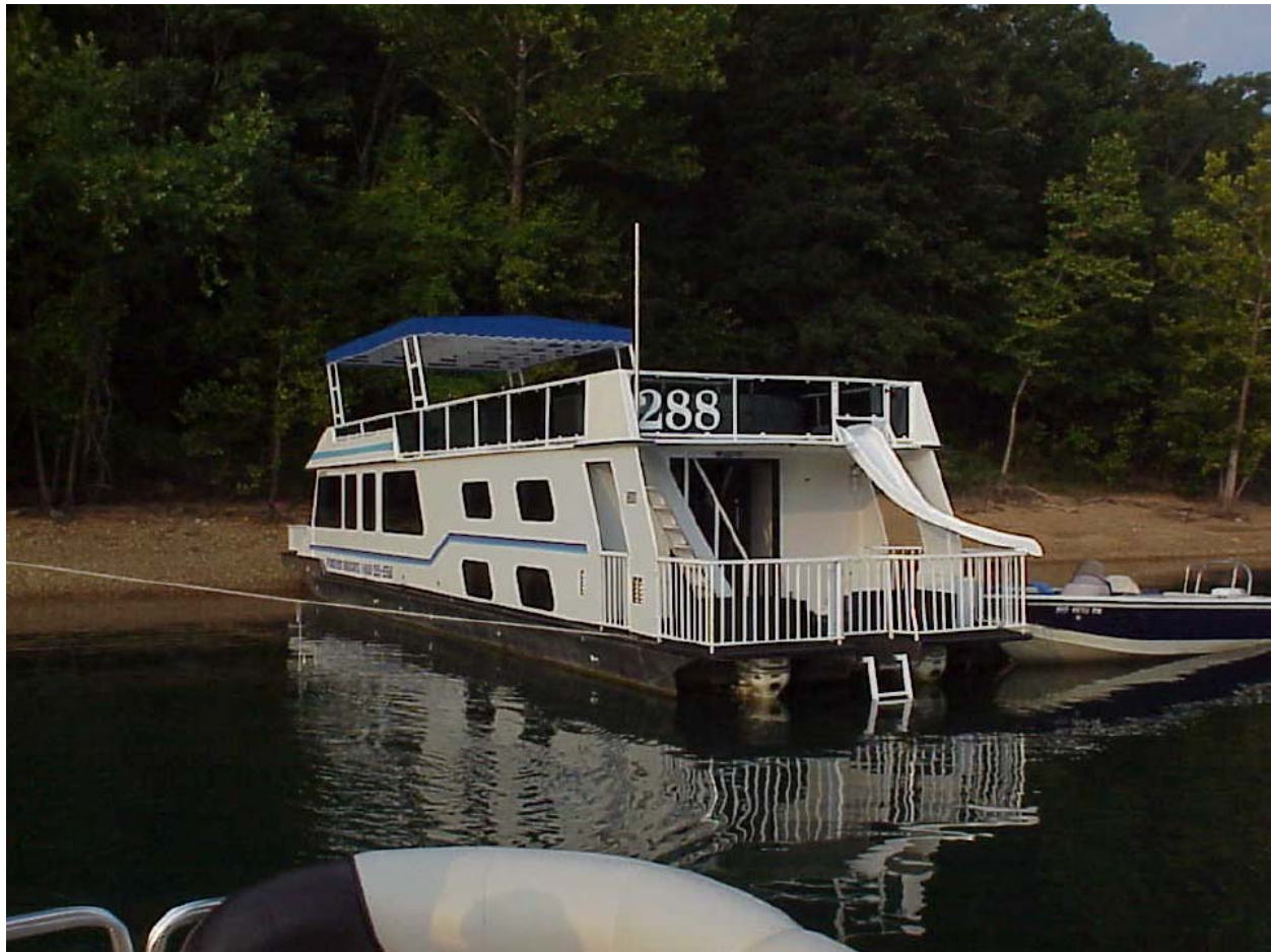
Figure 1. Houseboat #1. 2000 Fun Country Marine Houseboat with Vertical Exhaust Stack.
