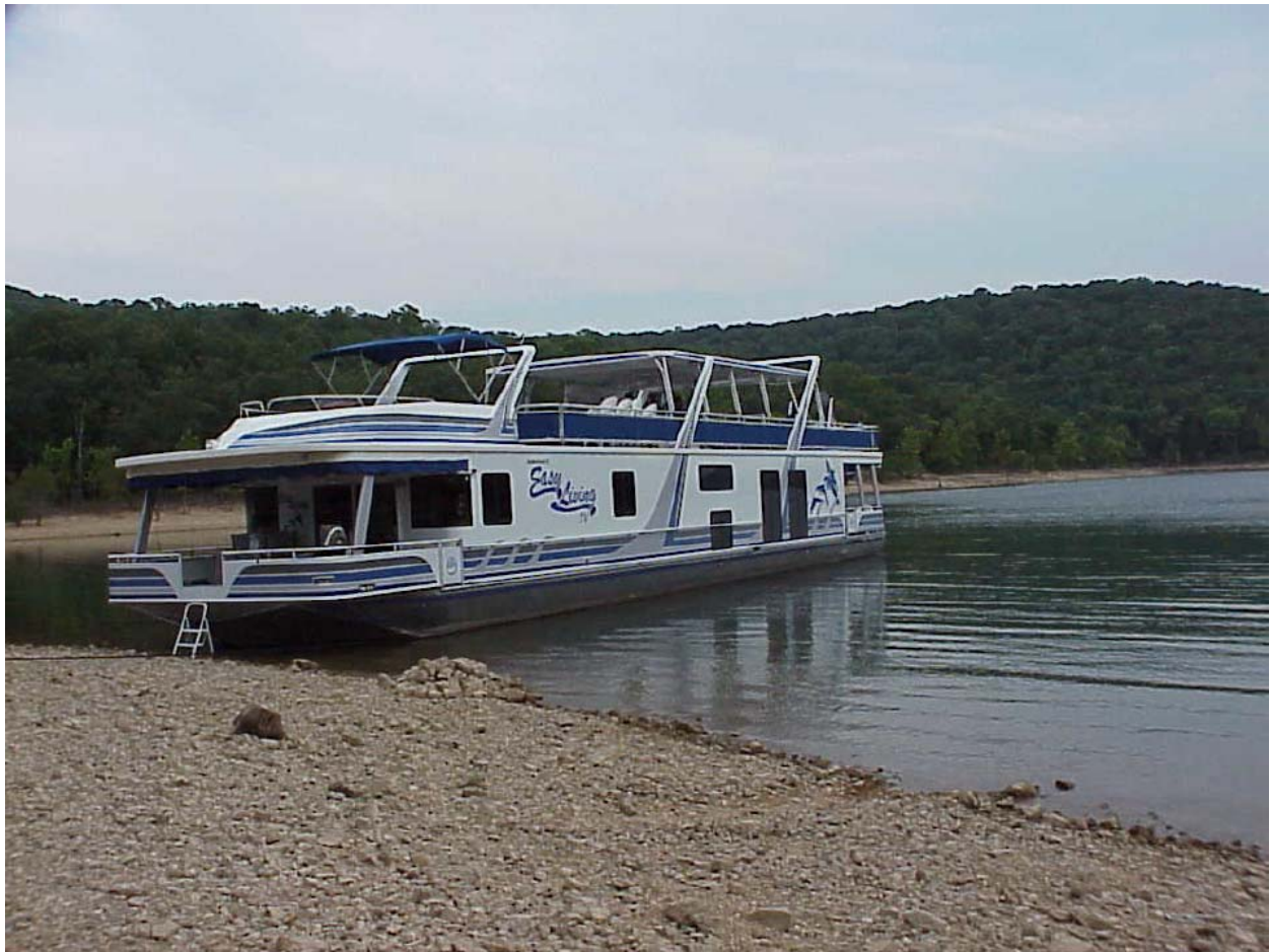
Figure 2. Houseboat #2. 2002 Somerset Houseboat with Flag Pole Exhaust Stack.
