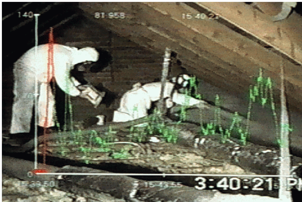
Appendix F – Picture 6. Example of finished Video Exposure Monitoring to observe employee activity and the associated total dust concentration (Real-time Monitoring also conducted – left).
