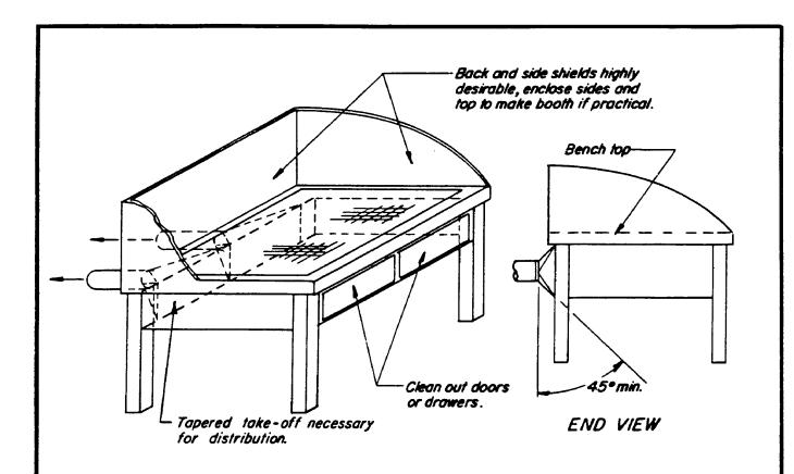
Q = 150 - 250 cfm /sq ft of bench area. Minimum duct velocity = 3500 fpm Entry loss = 0.25 VP for tapered take-off.
