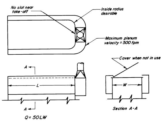
Slot velocity = 1000 fpm maximum Entry loss =1.78 slot VP + 0.25 duct VP Duct velocity = 2500-3000 fpm
